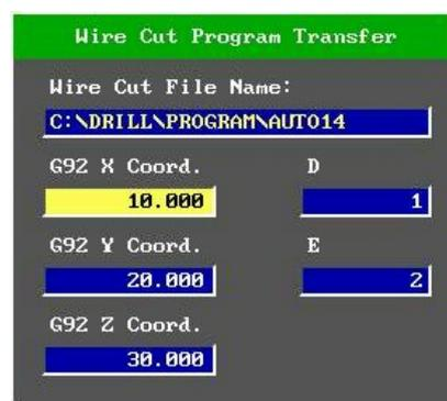
Figure 4-4-6 the transferring Wire Cut Program Frame
