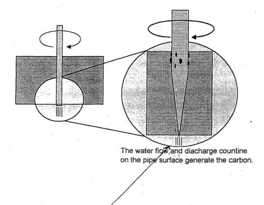
P.S When user find the pipe not easy and take time to drilling near finished holes the user can use a plastic bar to touch the drilling hole point let pipe easy pass through the hole.
