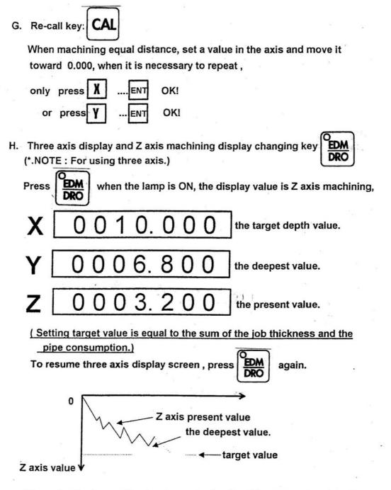
If target value is equal to the deepest value, it will output a signal to stop "discharge".
