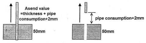
The upward speed adjust "speed feedrate".
