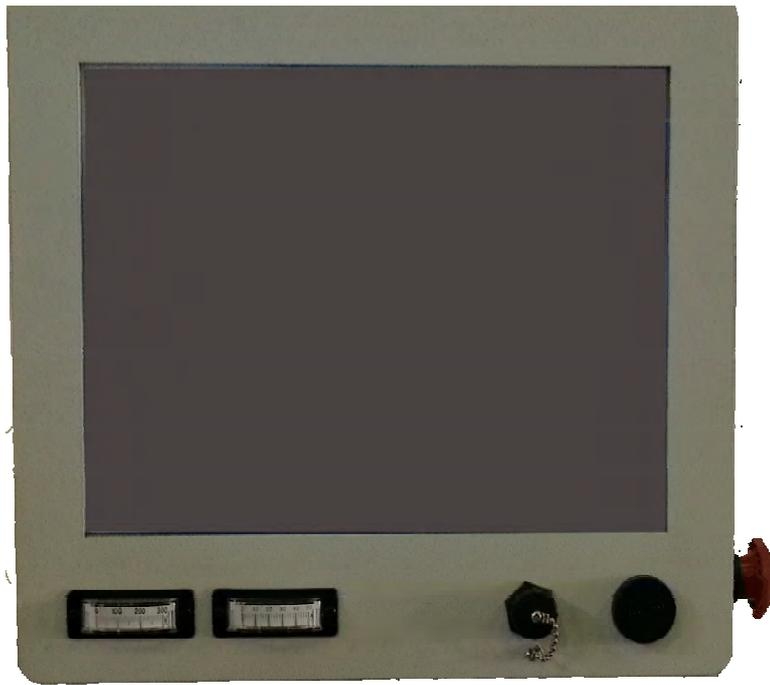
Figure 1-1-1 LCD Touch display panel
