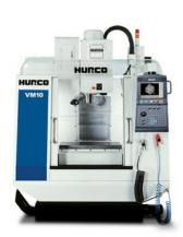
The VM10 is the fastest growing vertical machining centre in the UK because of its perfect combination of size and functionality. It has the smallest footprint and large capacity for efficient machining and productivity. Machine is fitted with full Hurco options including NC merg and Renishaw Probing. The 660x406x508 mm work envelope in a 1.8x1.6m working footprint makes the VM1 very attractive for most applications.
