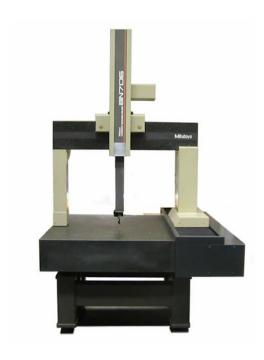
Travel axes (X x Y x Z): 700 x 600 x 450 mm
